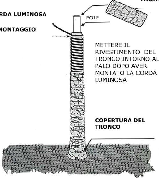
METTERE IL RIVESTIMENTO DEL TRONCO INTORNO AL PALO DOPO AVER MONTATO LA CORDA LUMINOSA
